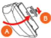
Figure 9 – Attaching the mounting bracket to the AP
