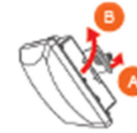
Figure 6 – Removing the mounting bracket
