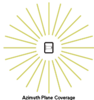
Figure 2 – Typical AP internal omni coverage, top view
