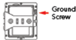
Figure 11 – Connect good earth ground to the AP here
